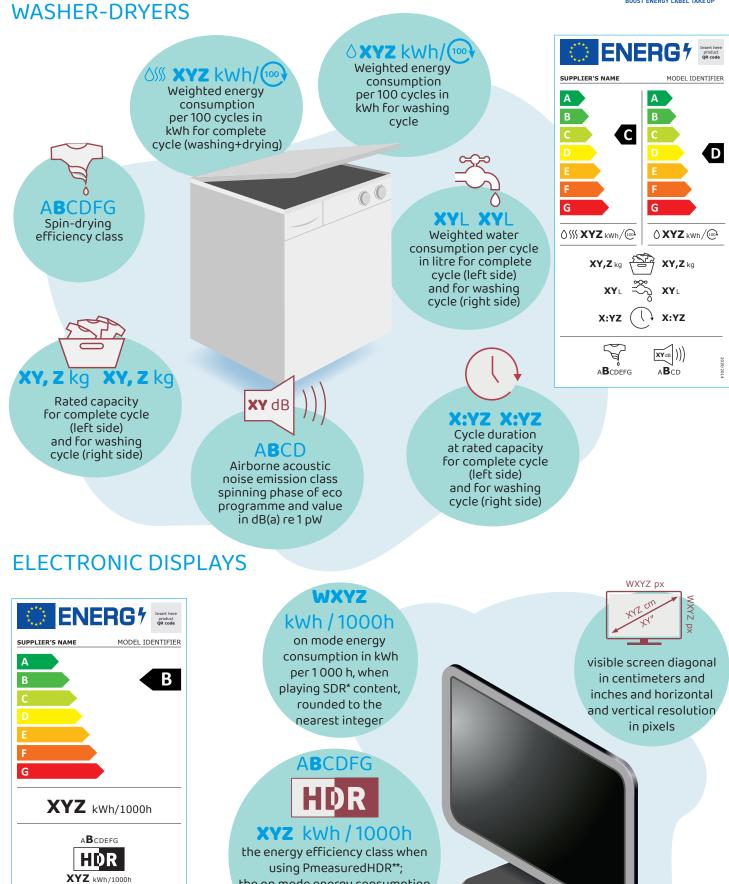
using PmeasuredHDR\*\*; the on mode energy consumption in kWh per 1 000 h, when playing HDR content, rounded to the nearest integer
